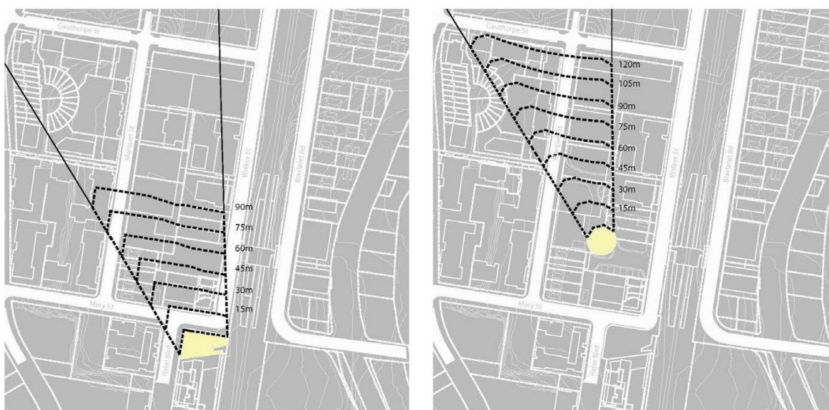
Figure 10: Solar Access Planes (defining potential heights of buildings in relation to areas where solar access must be either fully protected, i.e. Town Square, or maximised i.e. child care centre, mid-block plaza and laneways).
