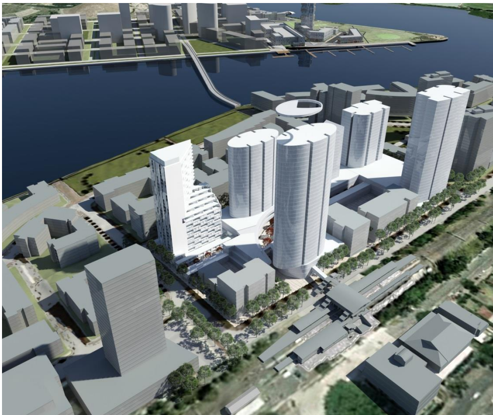
Figure 9: Station Precinct Master Plan - perspective based on 3D computer modelling (showing built form, including laneways, podium shapes, tower locations, heights and indicative heliostat structure).
